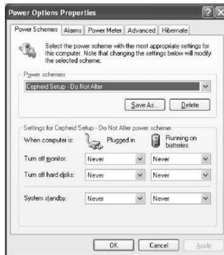
Gambar 4.8 Tampilan kotak dialog Power Options Properties, Tab Power Schemes (Sumber: GeneXpert® Operator Manual, Cepheid)
