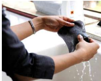
Gambar 6.8 Cara mencuci filter debu kipas alat TCM
